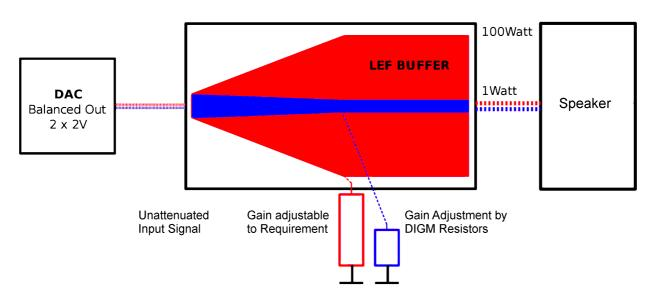
Red = High volume: The unattenuated input signal of 4V is amplified about 7 times. Blue = Low volume: The unattenuated input signal of 4V is amplified about 0.7 times.
