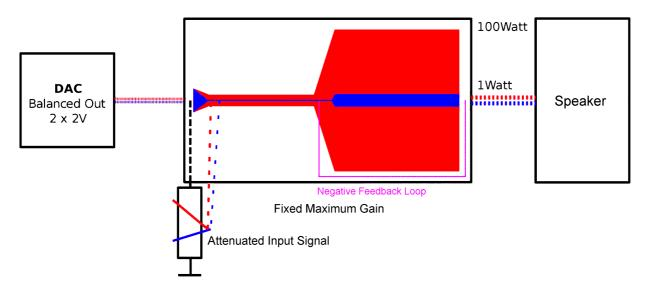
Red = High volume: The input signal is reduced from 4V to less than 1V, then amplified about 30 times.
