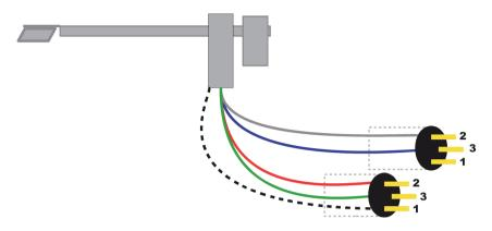
The attached direct wiring is generally the best interconnection with the least contact transitions. An optimum sound quality requires an excellent sounding interconnection.
