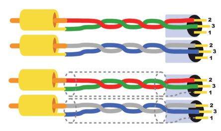
For RCA to XLR connection it is essential to ensure that the RCA "ground" has no connection to the XLR-ground (pin 1)! Reminder: RCA in this case has no ground!
