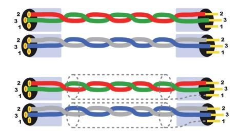
XLR to XLR is a standard balanced connection. However, here is something special: As a floating balanced connection, it does not need any ground connection, just non-inverting and inverting signals.
