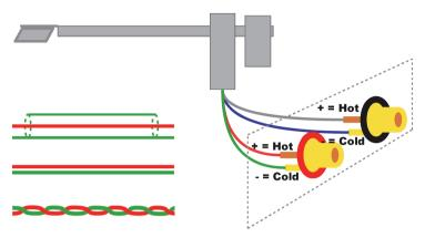
Within a record player balanced cables should be used, even if they end in RCA jacks. Coaxial cables should be replaced if possible.
