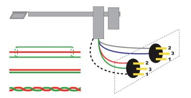
Within a record player balanced cables should be used. Coaxial cables should be replaced as far as possible.
