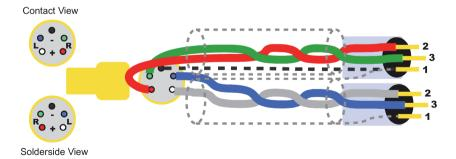
For the 5-Pin Tiffany to XLR connection is to be noted particularly that the tonearm ground is connected from the middle pin of the Tiffany-plug only to ONE channel XLR pin 1, otherwise risking hum noise due to a ground loop.
