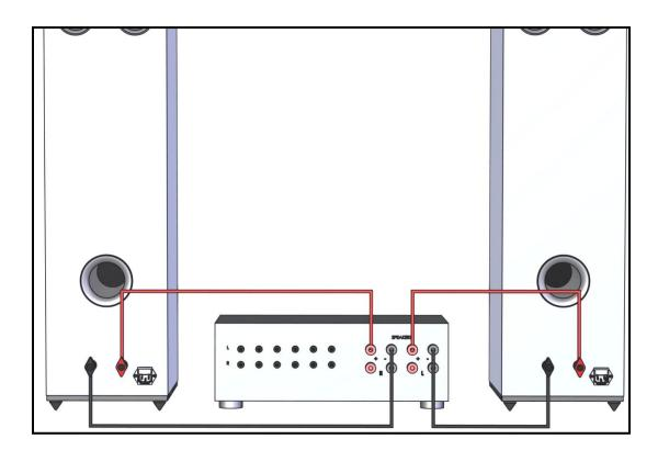
When connecting speaker cables, it is absolutely necessary to check for proper polarity: plus to plus and minus to minus. The screw clamps on the loudspeakers as well as the connectors on the amplifier are colour coded and labelled (positive pole = red, negative pole = black). To ensure proper connections, the wires on most speaker cables are also differentiated by colour, form, or marking. Reversing the polarity of the right and left channels results in sound distortions
