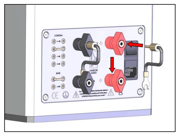
There are 2 cable bridges supplied for each speaker. When using a single wire connection use the bridges as shown on the previous page. This method allows for speaker cables terminated with banana plugs or spade lugs to be used.
