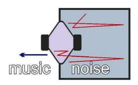
The composite diaphragm defeats the communication of internal reflections and other distortion that is unwanted energy acting against the music.
