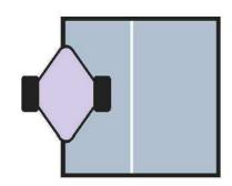
For a given limit of low frequency, the enclosure volume required by the Isobaric is half that of the single driver, conventional option.
