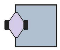
At 200 Hz and below the composite diaphragm is coupled and can be seen as a solid, super lightweight structure.
